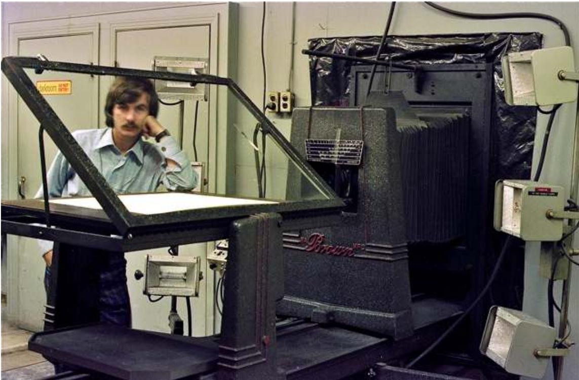
There were two large 18X24 offset or process cameras with vacuum backs in the darkroom. The darkroom had double light trapped doors. We worked under red safelights, as the film we were using was orthochromatic and not sensitive to red light. I started hand-developing film in open 20 X 30 trays of chemistry.
