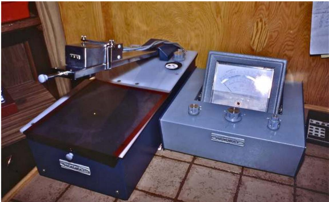
Exposure was done by a Ultraviolet contact printer and light source built from plans included in Luis Nadeau's books which utilizes 350nanometer bug bulbs.
