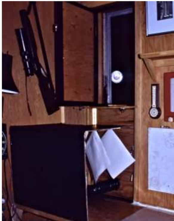
An enlarger was also needed for making enlarged negatives used in the process.
